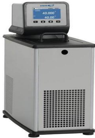
Fig. 2.4. Refrigerated circulating water bath with temperature controller that has an accuracy of \pm 0.1^{\circ}\text{C} .
