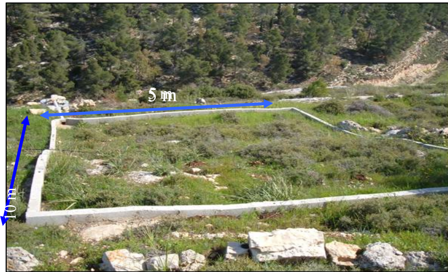
Fig. 1. Micro-catchment (50 m 2 ) with natural vegetation to collect runoff and sedimentation
