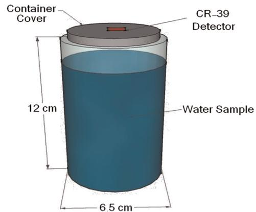
Fig. 2. Schematic diagram for measuring radon concentration in the water samples.
