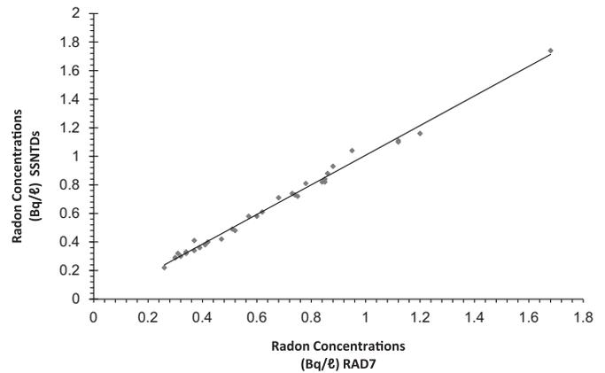
**Fig. 3.** The linearity between the results of two detectors; active (RAD7) and passive (SSNTDs).
