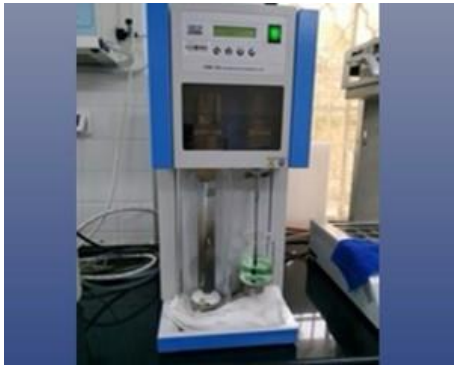
Figure 3.7: Distillation by using Kjeldahl and titration of the grape samples.
