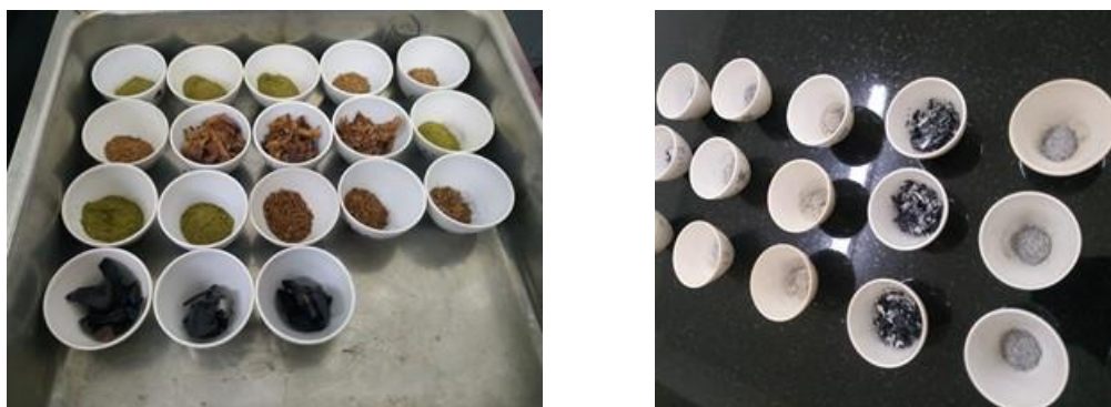
Figure 3.3: Grape samples before and after burning on a muffle furnace at 550 °C.
