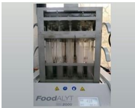
Figure 3.6: Digestion of the grape samples by using Foodalyt SBS 2000 system.
