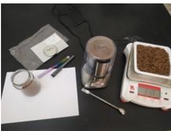
Figure 3.2: Preparation, crushing and storage of grape leaves and fruits.
