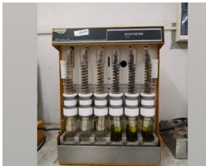
Figure 3.9: Fat extraction of grape samples by Soxtherm device using diethyl ether.
