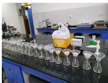
Figure 3.4: Filtration of the grape samples after extraction from ash.
