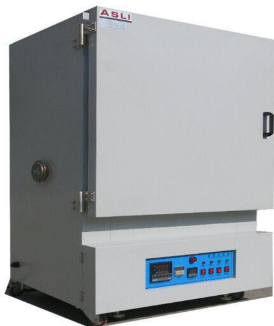
Figure 2.2. A Lab furnace by CM Furnaces with heating temperature up to 2000 K.
