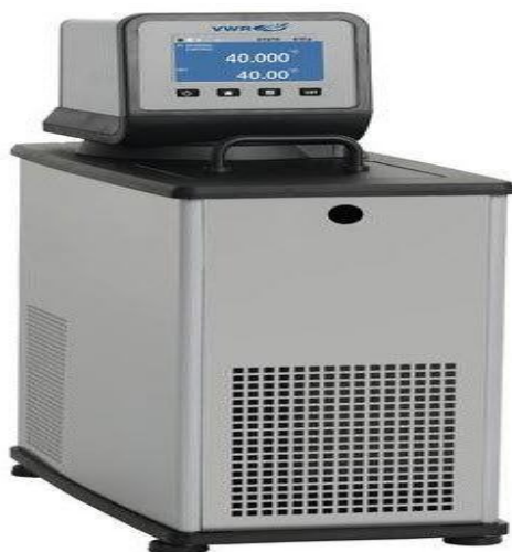
Figure 2.3. Refrigerated circulating water bath with temperature controller that has an accuracy of \pm 0.1^{\circ}\text{C} .
